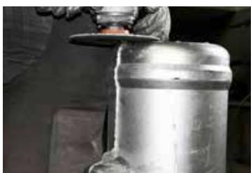
Grinding of cast parts
