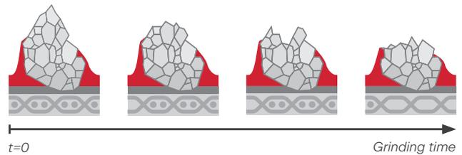
The microcrystalline structure of the **VSM CERAMICS** series enables a much more subtle breaking down of the grain and constantly produces new sharp edges.
